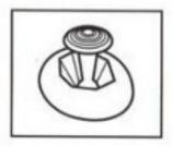
To reset the neutral position once the game has started, let go of the Control Stick so it can return to its center position (as shown in the picture on the left) then press **START** while holding the **L** and **R** buttons.
